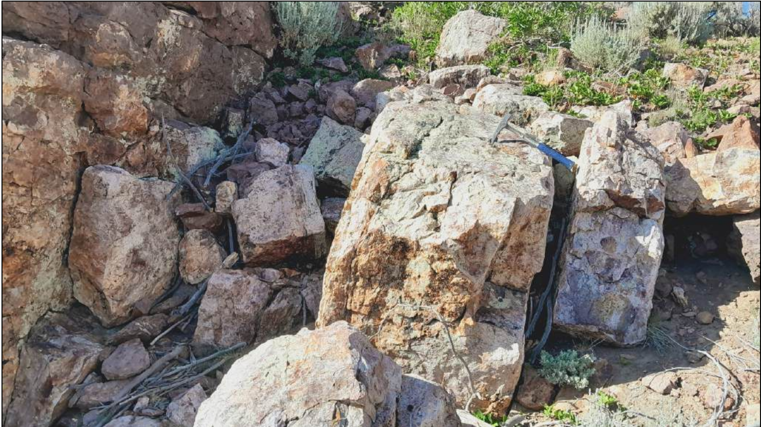
Outcrop of an approximately 2.7 metre-wide, southwest-striking vein. A selective sample from a 20 cm wide stage of green chalcidony returned 1.1 g/t gold and 52.6 g/t silver.
