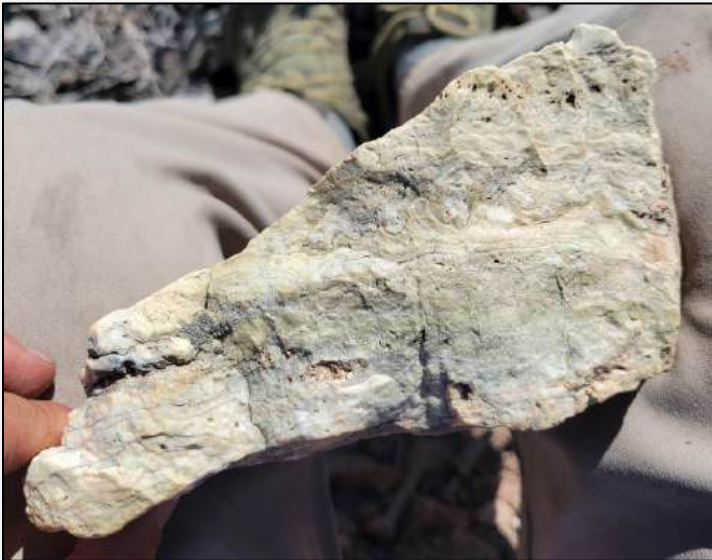
Fine-grained quartz vein float with crustiform-colloform banding. Returned 1.3 g/t gold and 49.7 g/t silver.
