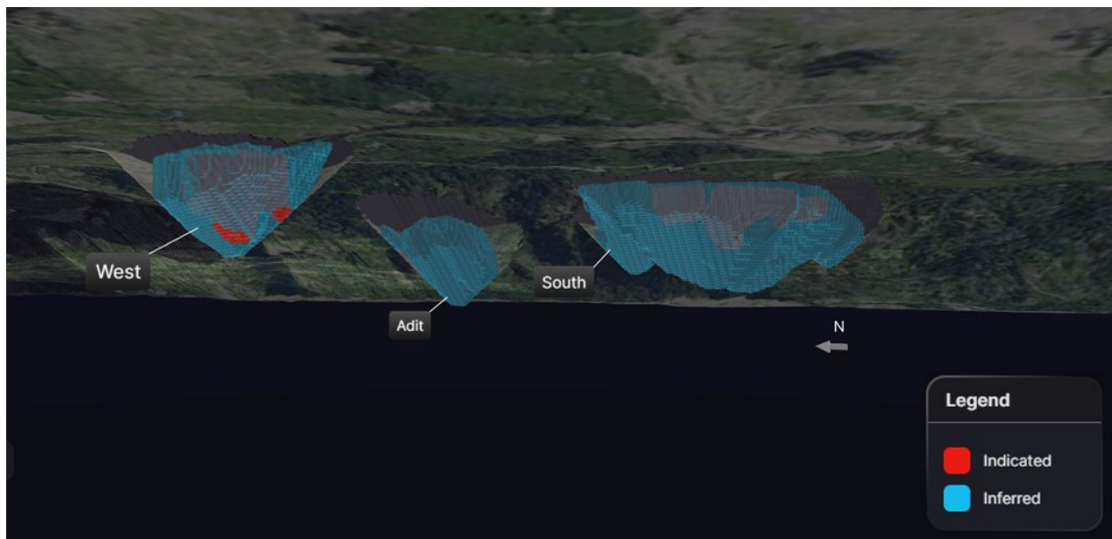
Figure 3 - MPD Project – Underground view of Mineral Resource Block Models and associated RPEEE 3D pit shells from Kodiak 1 .
