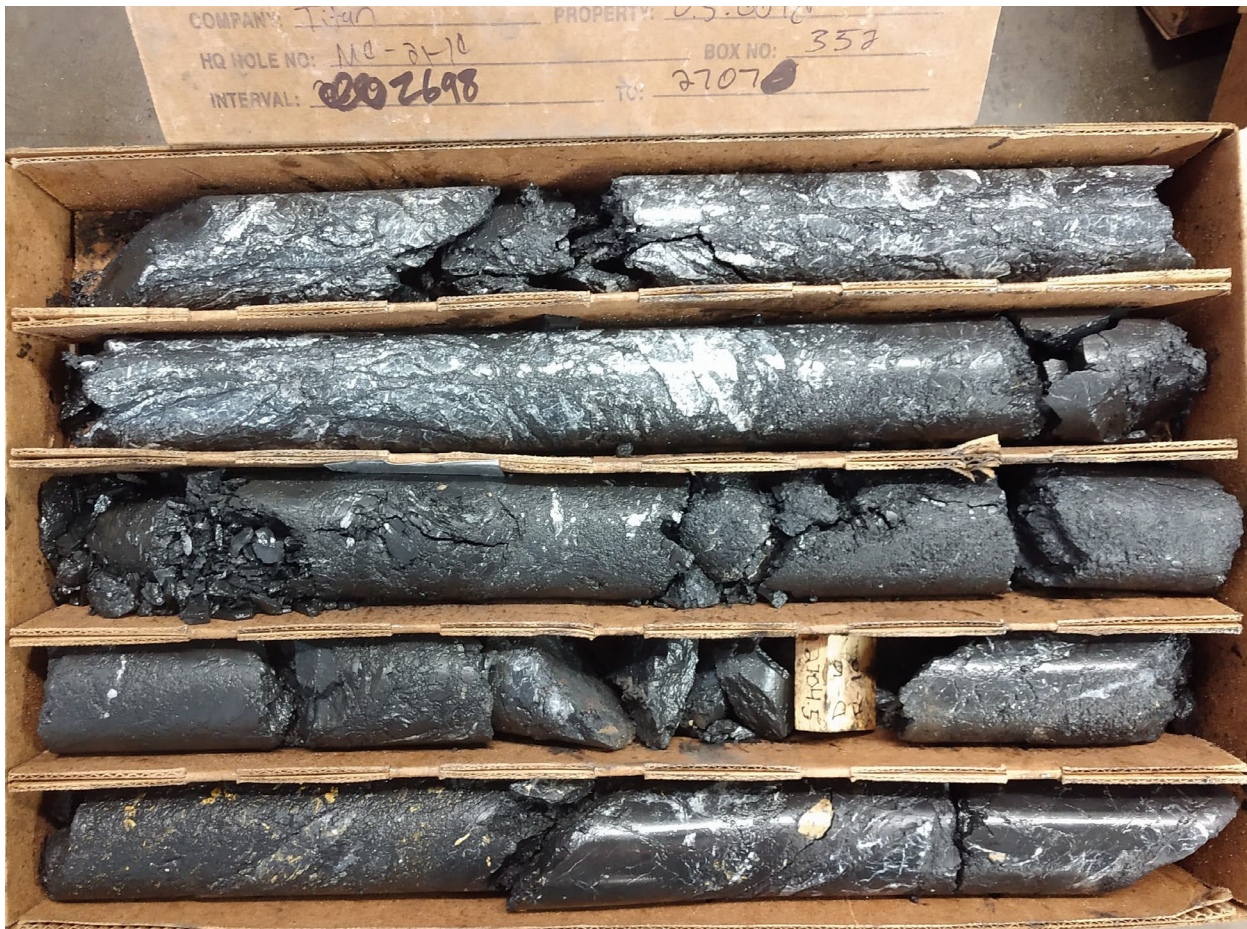
Photo 1. Brecciated, decalcified and dolomitized Wispy Member Popovich with sooty pyrite and orpiment.
