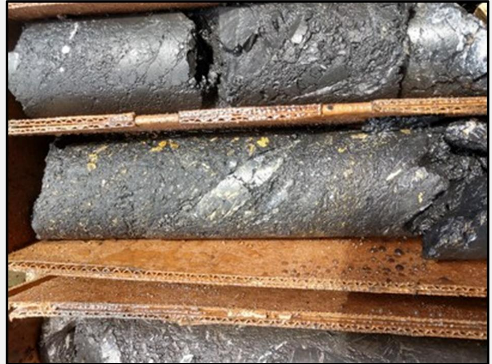
Orpiment and sooty pyrite in brecciated interval of Wispy Popovich formation with elevated gold (165 ppb) from MC21-1C
